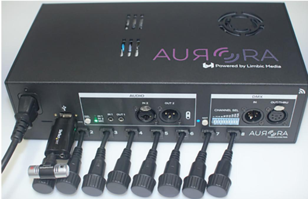
Fig. 29: USB Audio interface + 1/8" microphone connected to Aurora Pro
