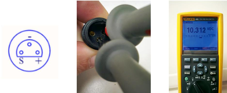
Figs. 40-42: Measuring end-of-line voltage
