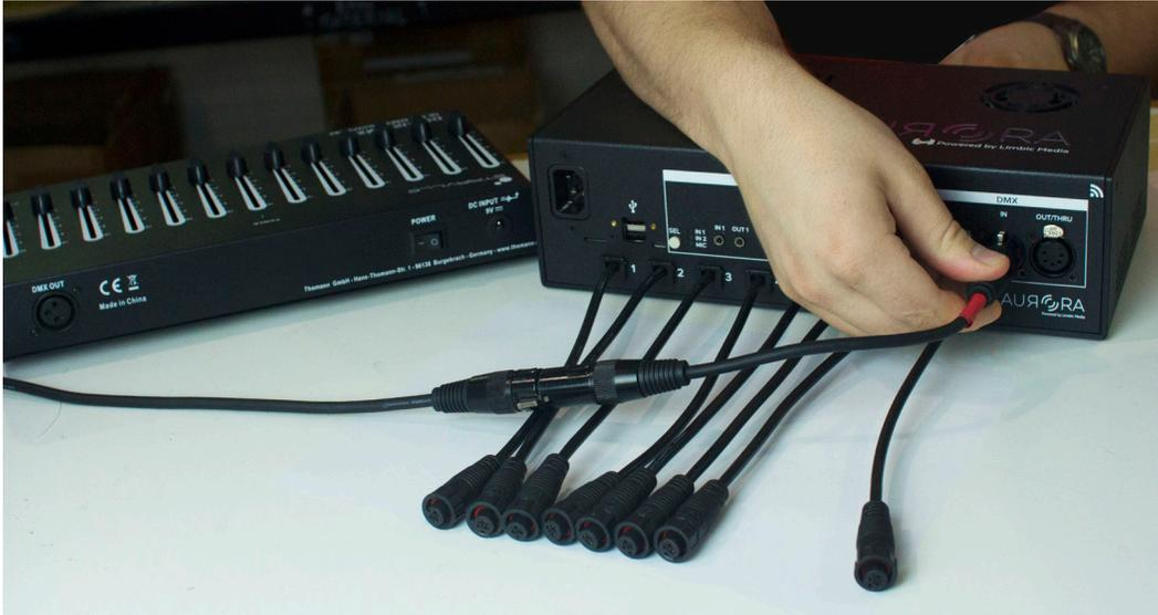
Fig. 33: Connect a DMX controller to Aurora Pro's 5-pin DMX IN port.
