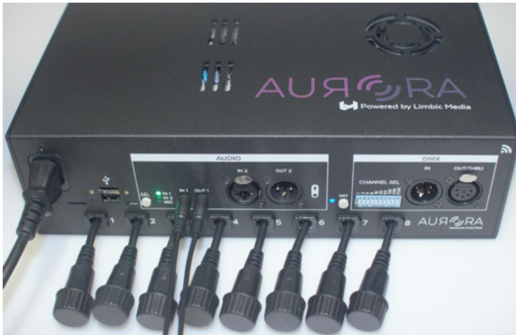
Fig. 26: Aurora Pro with 1/8" IN/THRU (IN 1 THRU 1) audio connected
