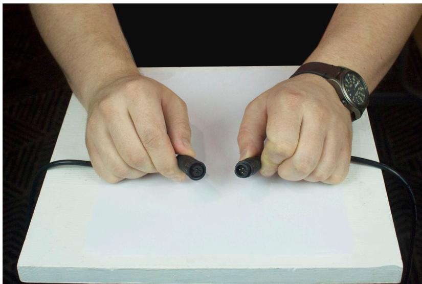
Fig. 2: Male and female ends of RGB connectors
